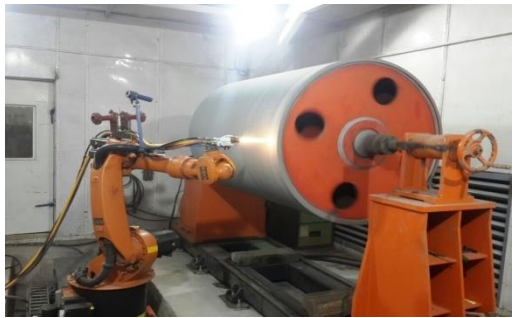
Acoustic spray booth for thermal spray coatings
