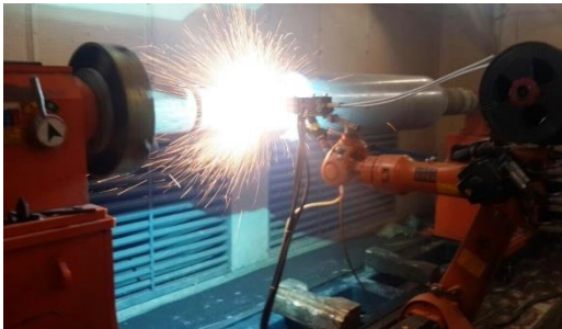
Dimensional Restoration of Bearing Journals
