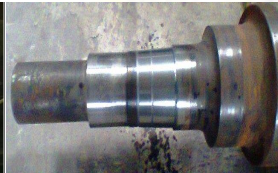
Journal Ground after repair
